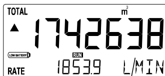
Fig. 3: Example of low-battery alarm.
